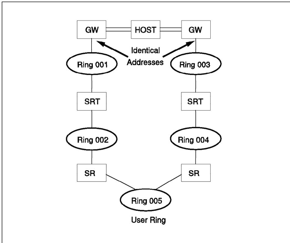
Figure 21. High-Availability Design and SRT. Equally, the SR and SRT bridge positions could be reversed.
