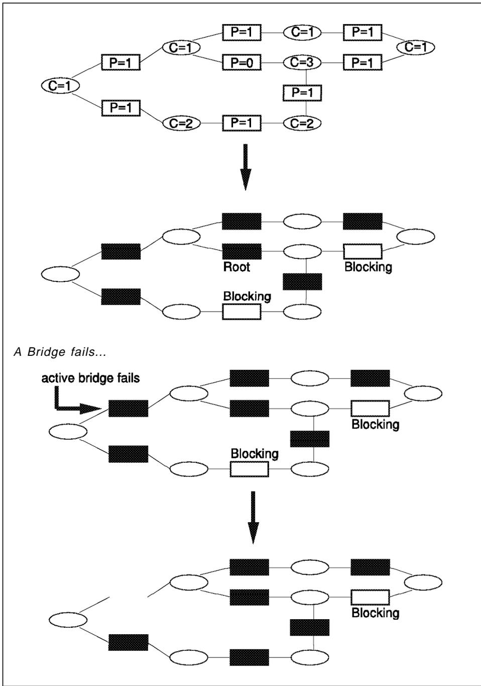
Figure 11. Reconfiguration of a Spanning Tree
