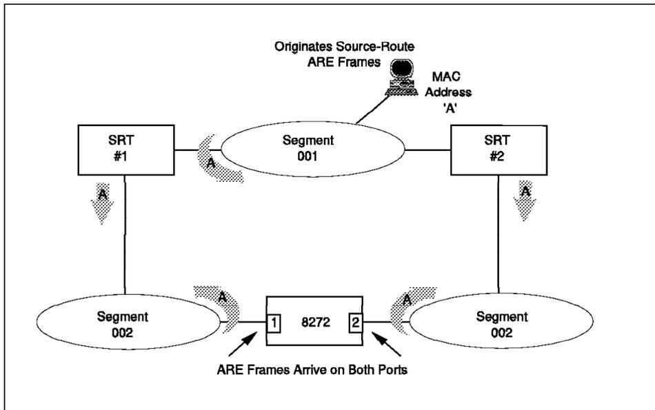
Figure 40. ARE Frames Passed by SRT Bridges
