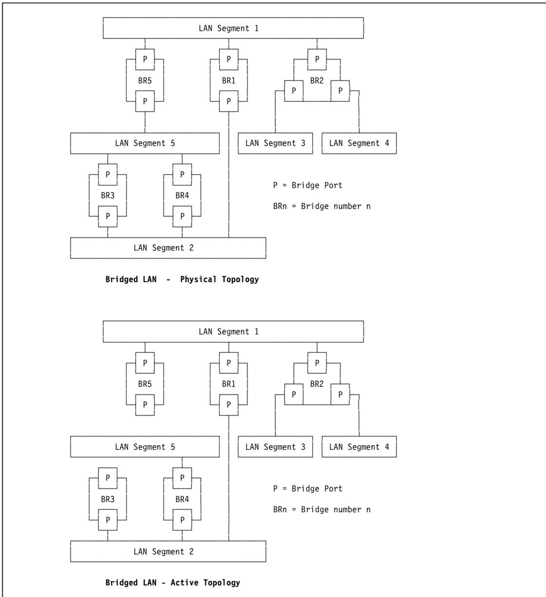
Figure 8. Example of Physical Topology. Also shown is a possible active Spanning Tree topology.
