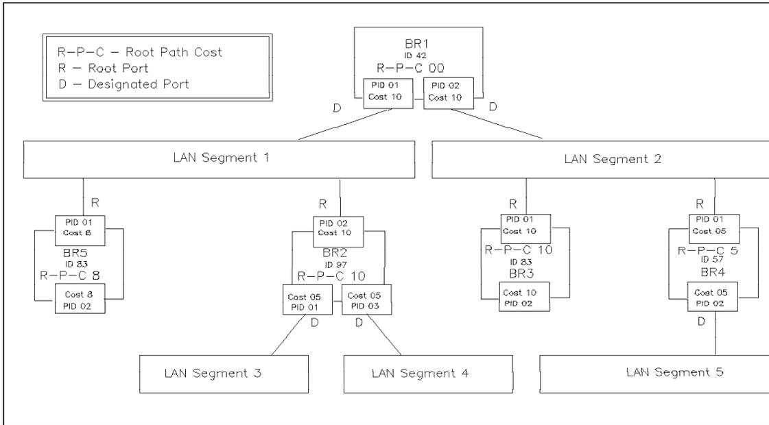
Figure 10. Bridged LAN - Logical Spanning Tree Topology
