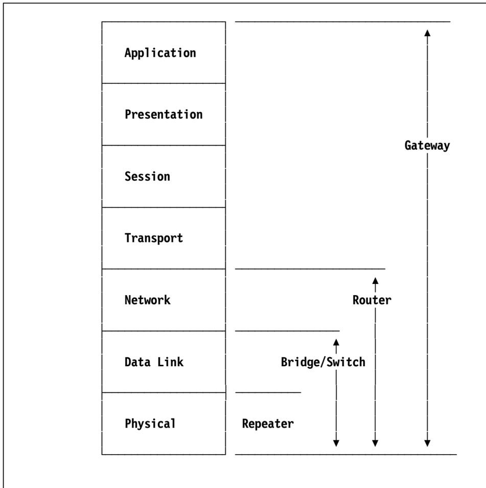
Figure 5. OSI Reference Model and Internetworking Devices
