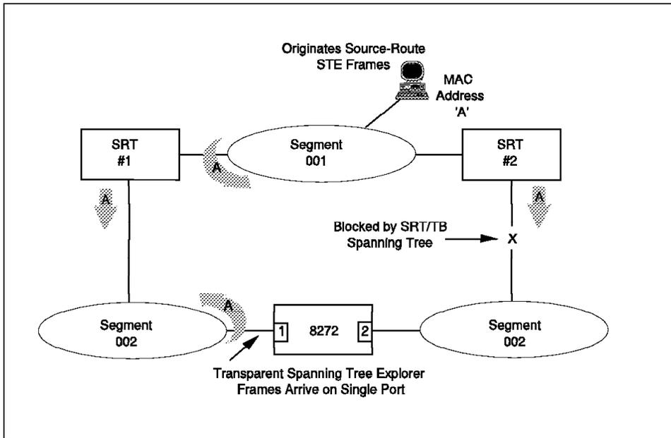
Figure 39. Blocked SRT Spanning Tree
